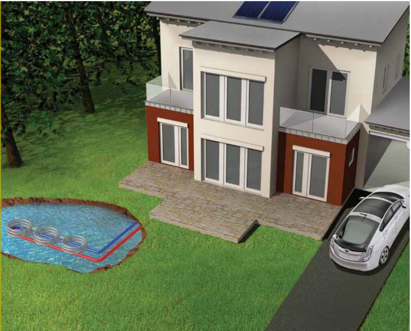
This type of design is economical when a project is located near a body of water. Fluid circulates through polyethylene piping in a closed system, just as it does through ground loops but in this case underwater. The pipes may be coiled in a slinky to fit more surfaces into a given amount of space. The lake needs to be a minimum size and depth depending on the load. Lake loops have no adverse impact on the aquatic system.
