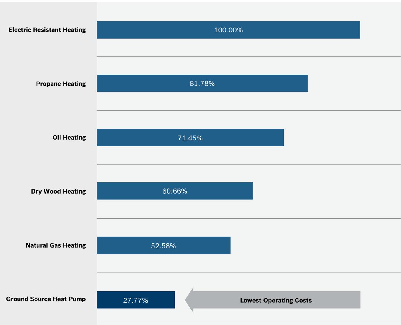
Estimated heating costs of operation for a building with 54,000 Btu/hr Design Heat Loss at -3 F.
