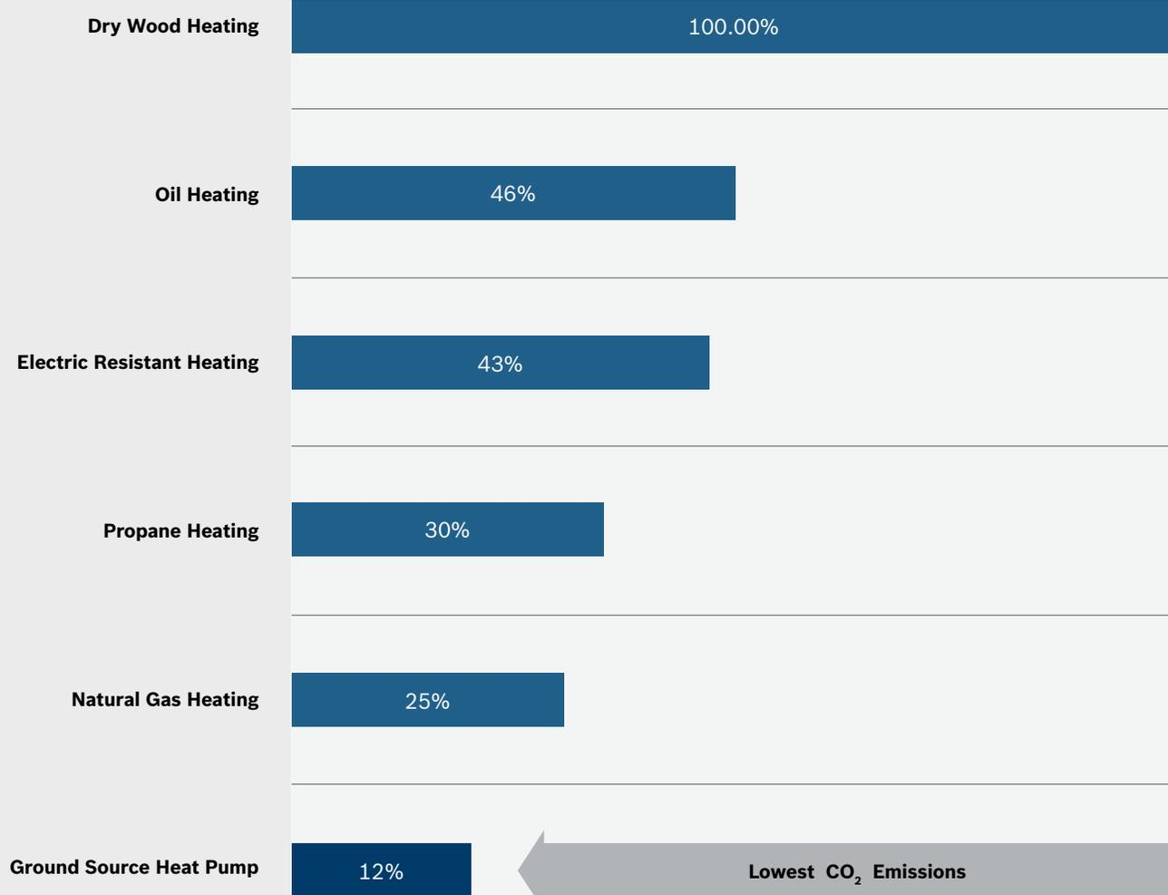
Estimated CO<sub>2</sub> emissions for a building with 54,000 Btu/hr Design Heat Loss at -3 F.
